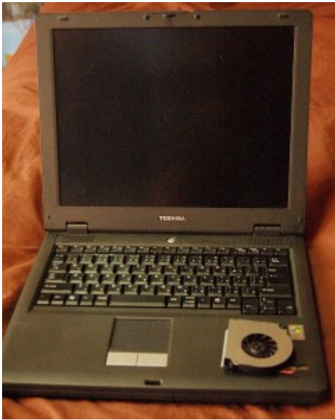
Toshiba Satellite J40. Broken CPU fan on the bottom right
